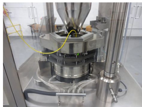
Dosing Station Manifold
